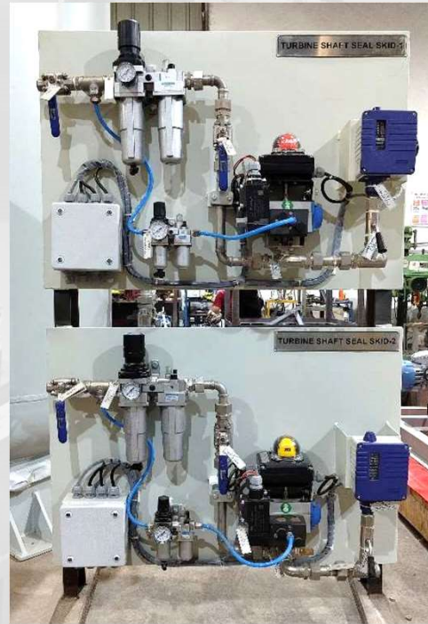
SHAFT SEAL PANELS
