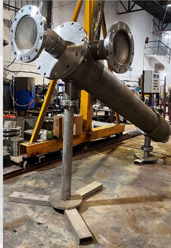
HYDRO CYCLONE SEPERATOR
